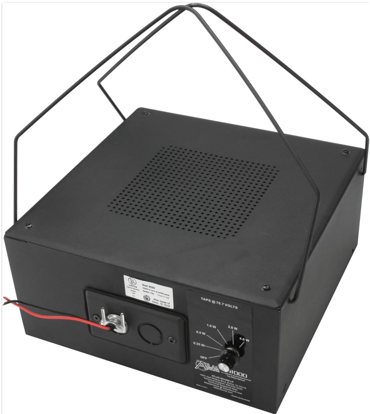
Figure 1: Atlas Sound M1000 speaker with visible tap selector switch and wiring input. The switch allows selection of power taps from 0.25W to 4.0W for 70.7V systems, or the 'OFF' position.
