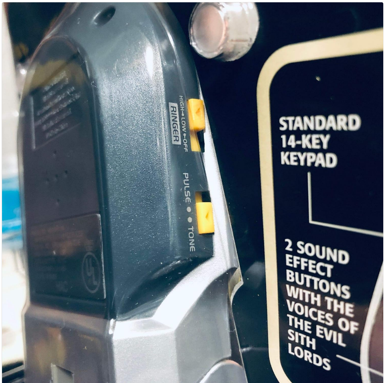
Figure 4.3: Side view showing the ringer (High/Low/Off) and Pulse/Tone switches.
