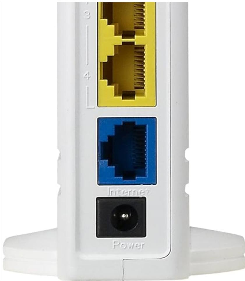
**Figure 2:** Rear View of the ASUS RT-N13U Router. This image displays the rear panel, including the USB 2.0 port, four LAN ports (yellow), one Internet (WAN) port (blue), and the power input port.
