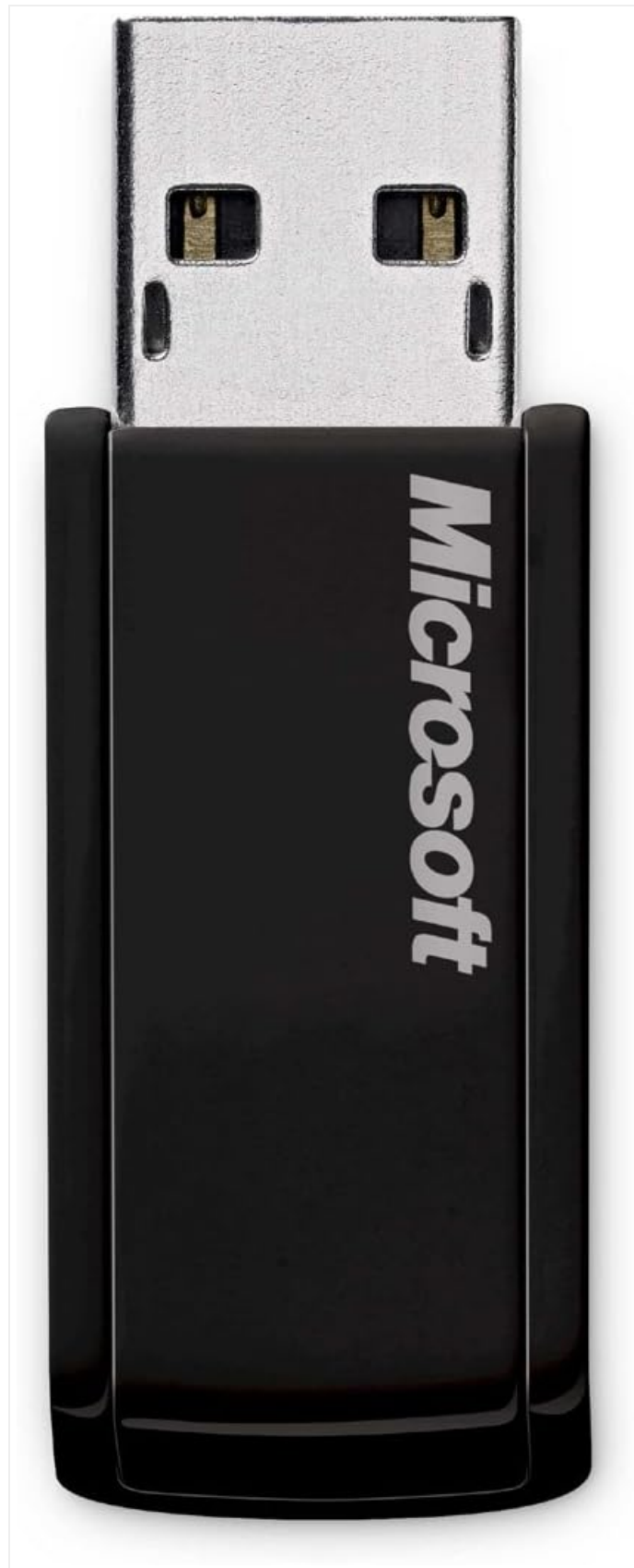
Figure 1: The compact USB mini-transceiver for wireless connection.
