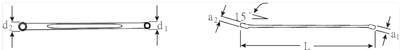
Figure 3.1: Technical drawing illustrating the dimensions of the Stahlwille 220 wrench, including length (L), head thicknesses (a1, a2), head widths (d1, d2), and the 15° angle.
