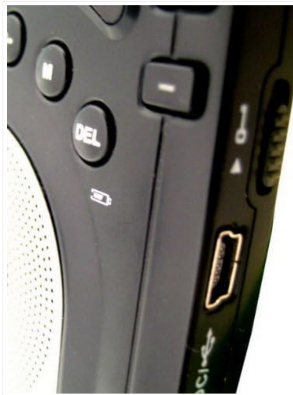
Figure 3: Detailed view of the side of the DEGEN DE15 radio, showing the earphone jack, USB port, and volume controls.
