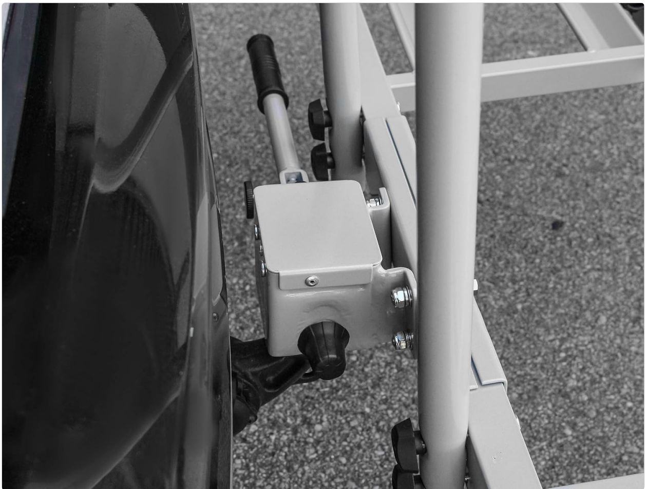
Figure 4.2: Rear view of the EUFAB 11402 Quick Lock Single attached to a bicycle carrier, demonstrating its position relative to the vehicle.
