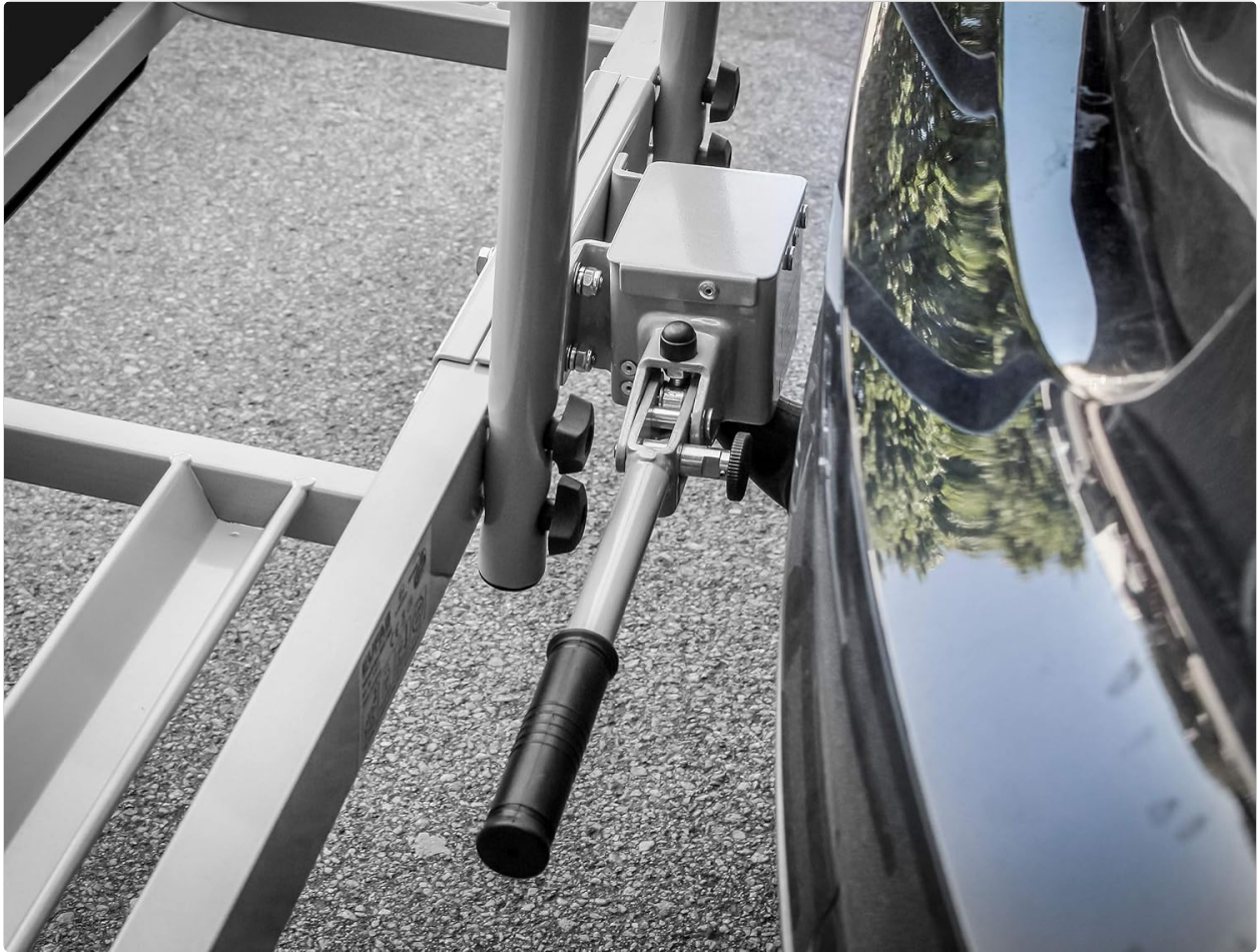
Figure 4.1: Side view of the EUFAB 11402 Quick Lock Single integrated into a bicycle carrier, ready for towbar attachment.
