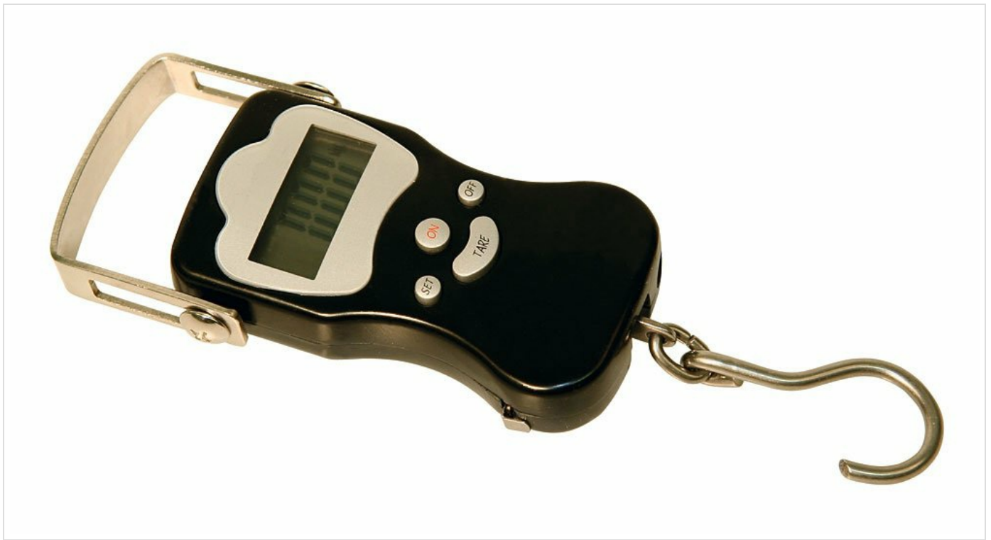
Image 1: Front view of the KERBL DigiScale 50, showing the digital display, ON/OFF, TARE, and SET buttons, and the hanging hook and handle.
