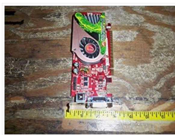
Figure 1: VisionTek ATI Radeon X1300 Low Profile Video Card. This image shows the compact design of the video card, highlighting its fan, heatsink, and DMS-59 connector. A ruler is visible at the bottom for scale.
