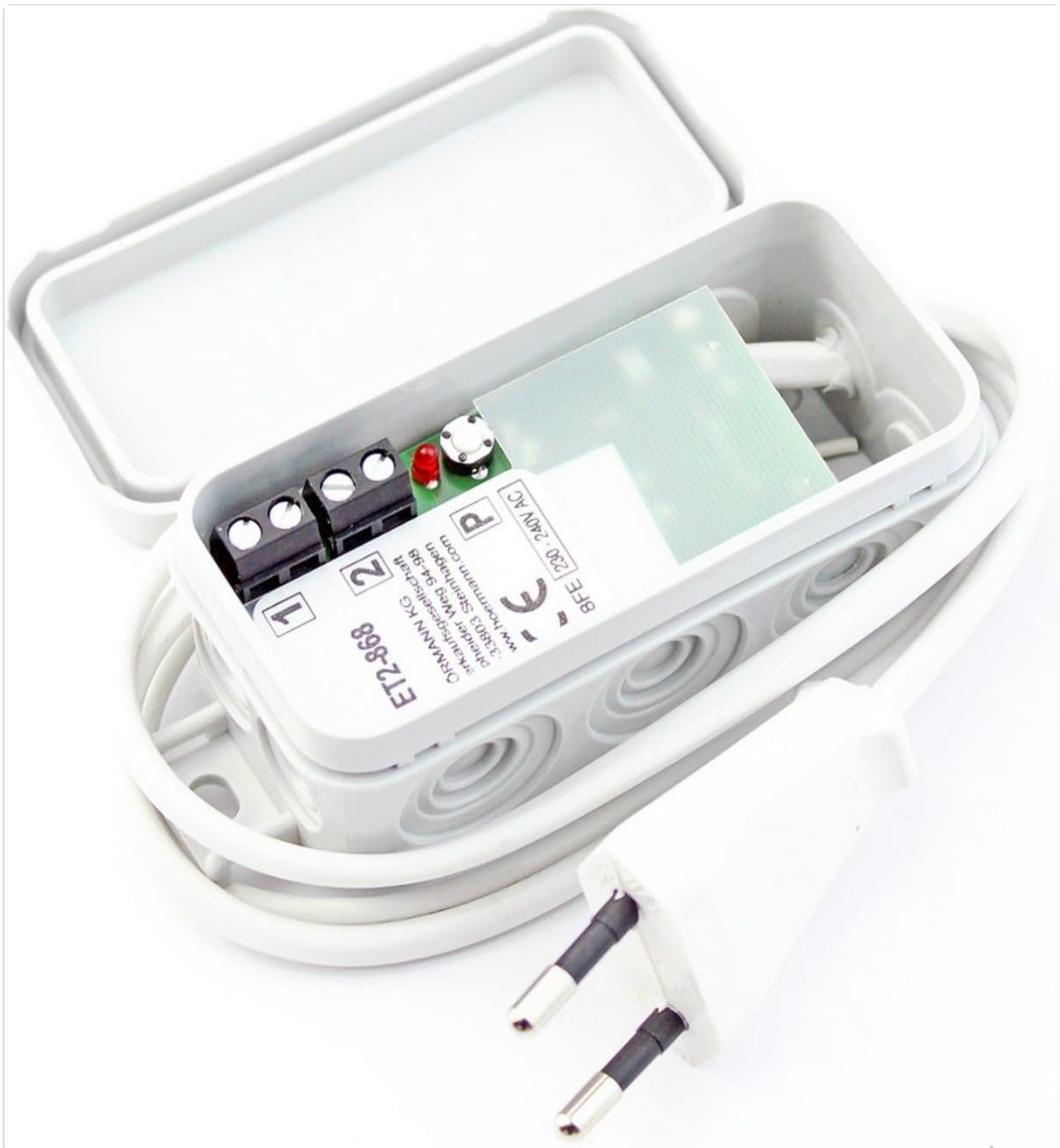
Figure 2: Internal view of the receiver showing wiring terminals. Connect the control wires to terminals 1 and 2 for the two potential-free relays.
