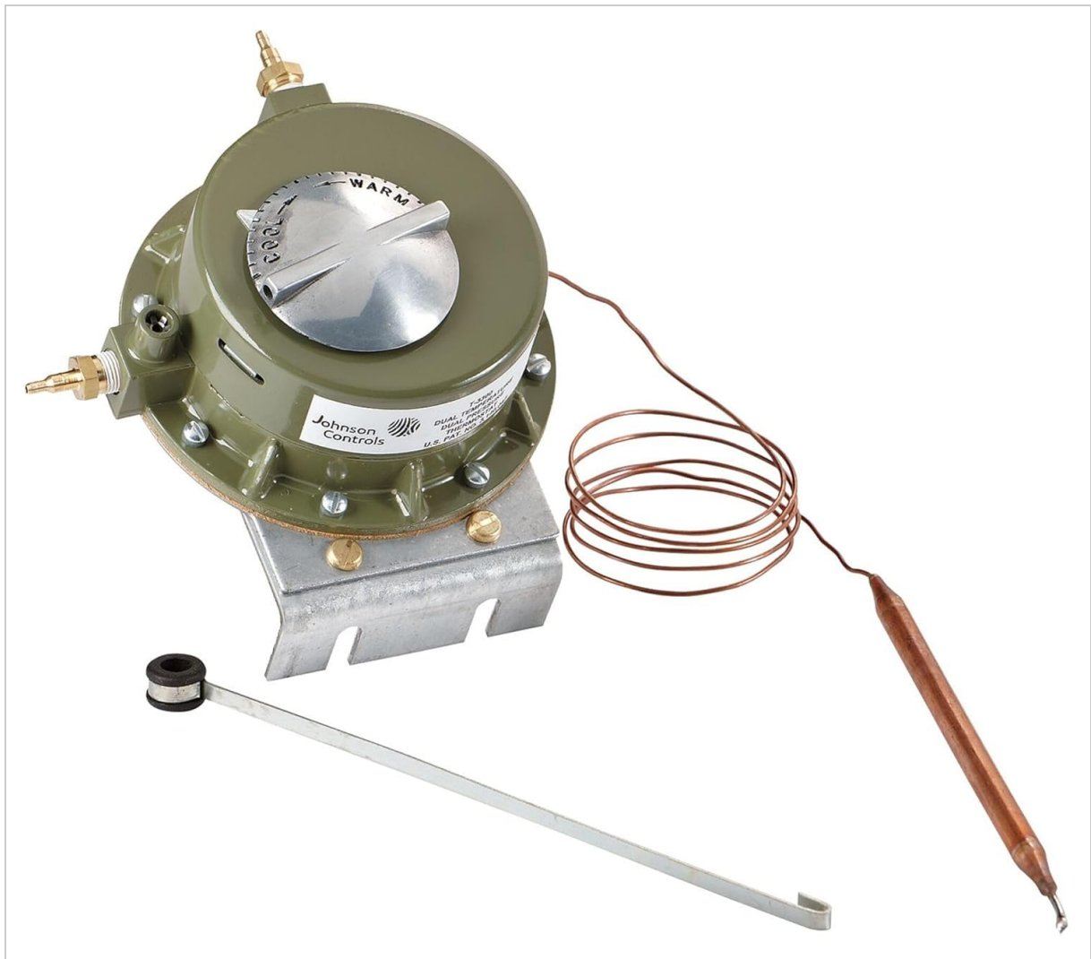
Figure 1: Overview of the Johnson Controls T-3300-1 Pneumatic Thermostat. The image displays the olive-green main control unit with a silver adjustment dial labeled 'COOL' to 'WARM'. Two brass pneumatic connections are visible on the top and left side. A coiled copper capillary tube extends from the unit, terminating in a copper temperature sensing bulb.
