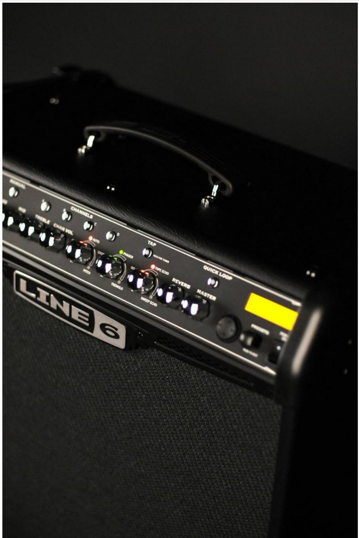
Image: Close-up of the Line 6 Spider IV 75 amplifier's control panel, detailing the amp model selection (Clean, Crunch, Metal, Insane) and the Drive, Bass, Mid, Treble, and Channel Volume knobs.
