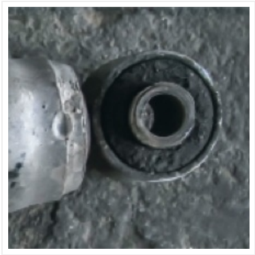
Image 6.1: A close-up view of a shock absorber bushing, illustrating a component that should be regularly inspected for wear and tear during maintenance checks.
