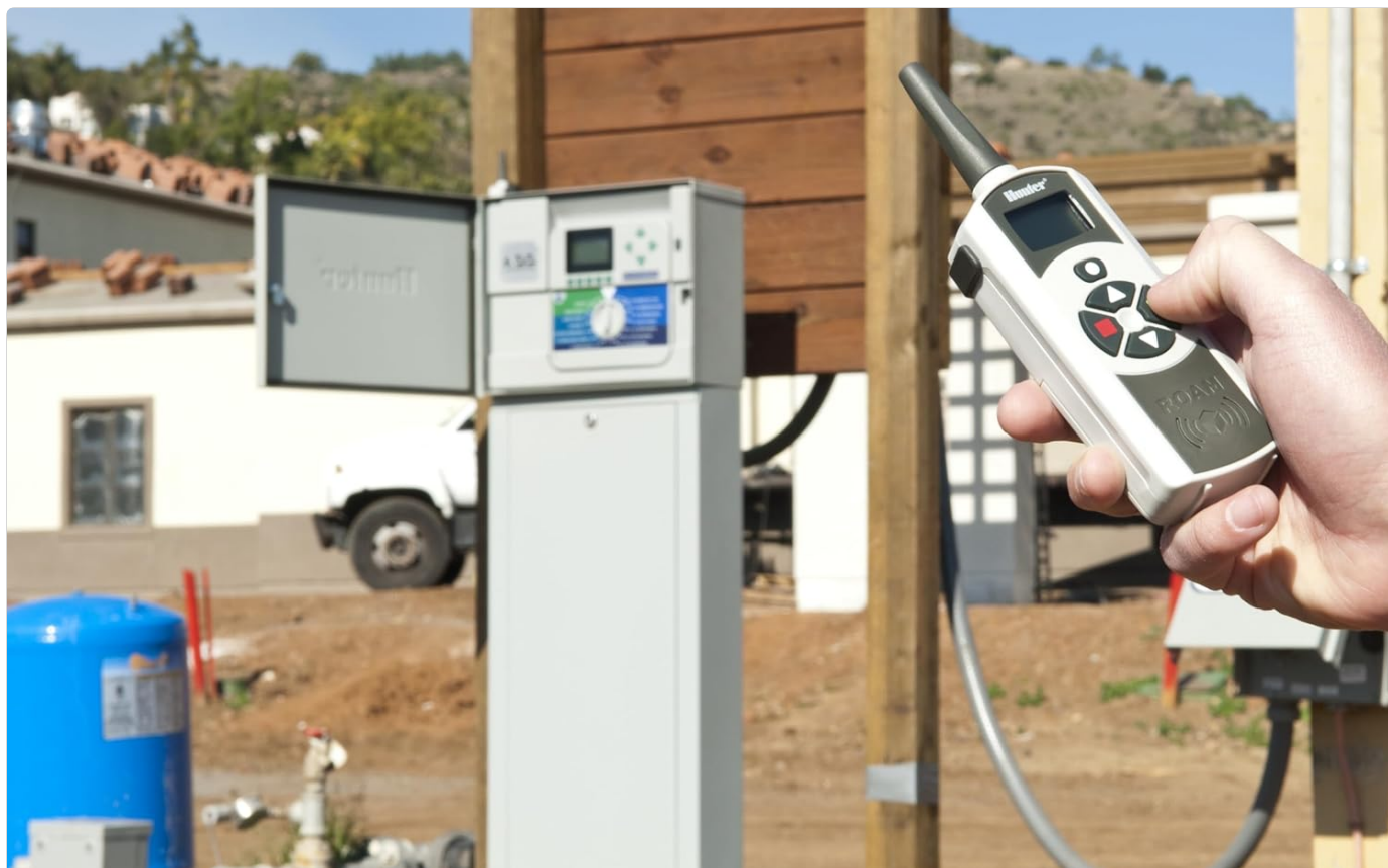
Image 2.3: Illustrates the connection of the SmartPort wiring harness to a Hunter irrigation controller.
