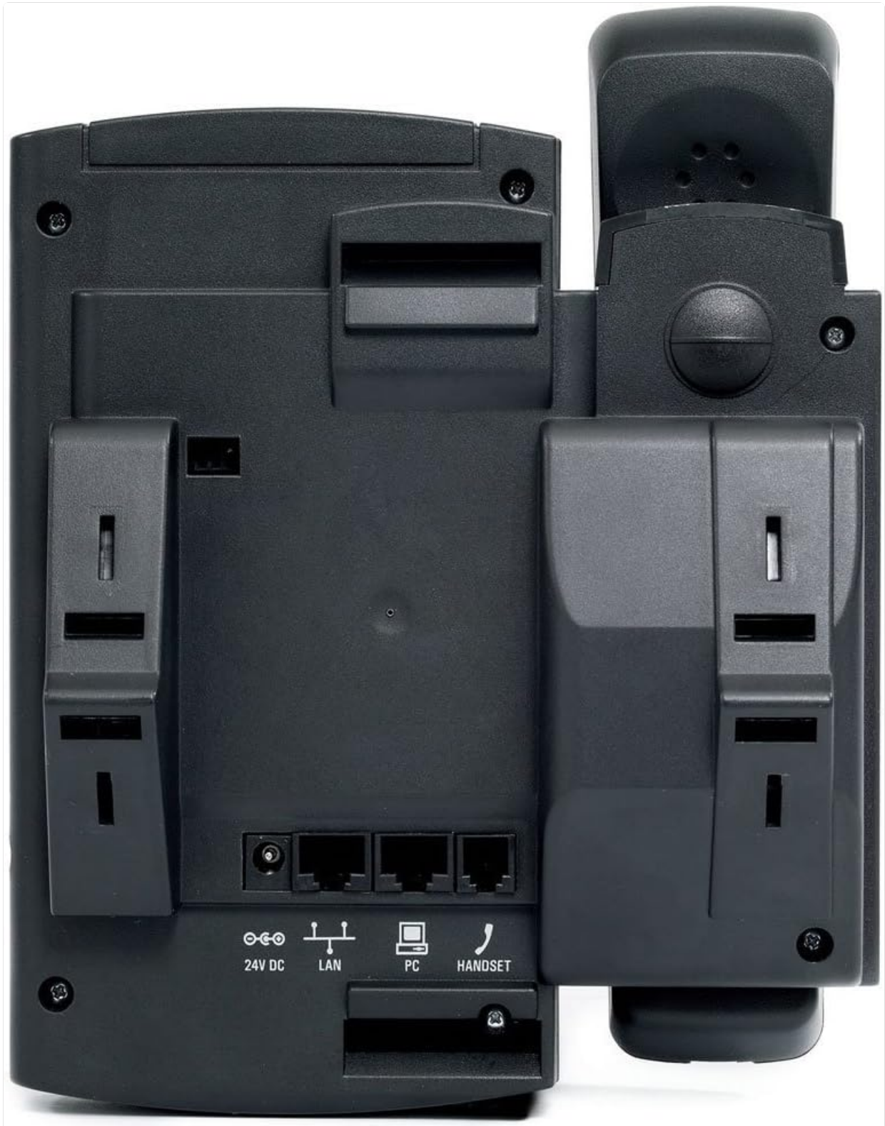
Figure 3.1: Rear view of the phone displaying the 24V DC power input, LAN port, PC port, and Handset port.
