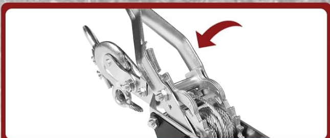
6 Lift the handle upwards to release the handle load
