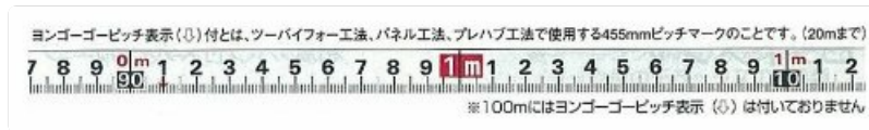
Figure 5: Close-up view of the tape showing the Yonggo pitch display, which marks 455mm intervals for specific construction applications.
