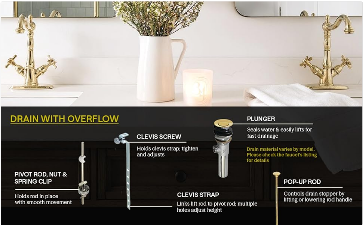
Image 3.1: Diagram illustrating the components of a typical pop-up drain assembly, including the pivot rod, nut, spring clip, clevis screw, clevis strap, plunger, and pop-up rod. This diagram helps identify parts for drain installation.
