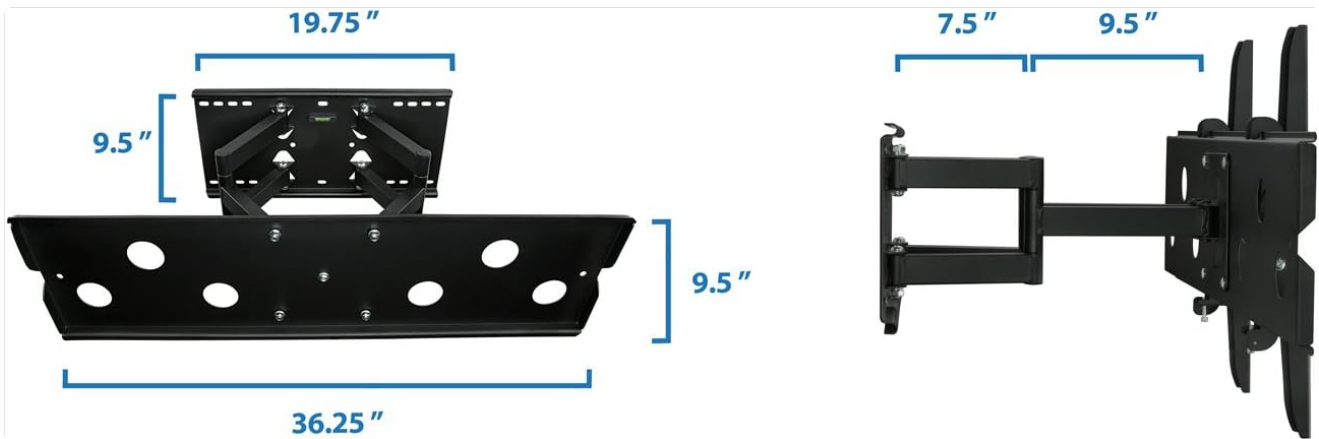
Figure 4.1: Wall plate and arm dimensions for planning installation. Wall plate is 19.75 inches wide.
