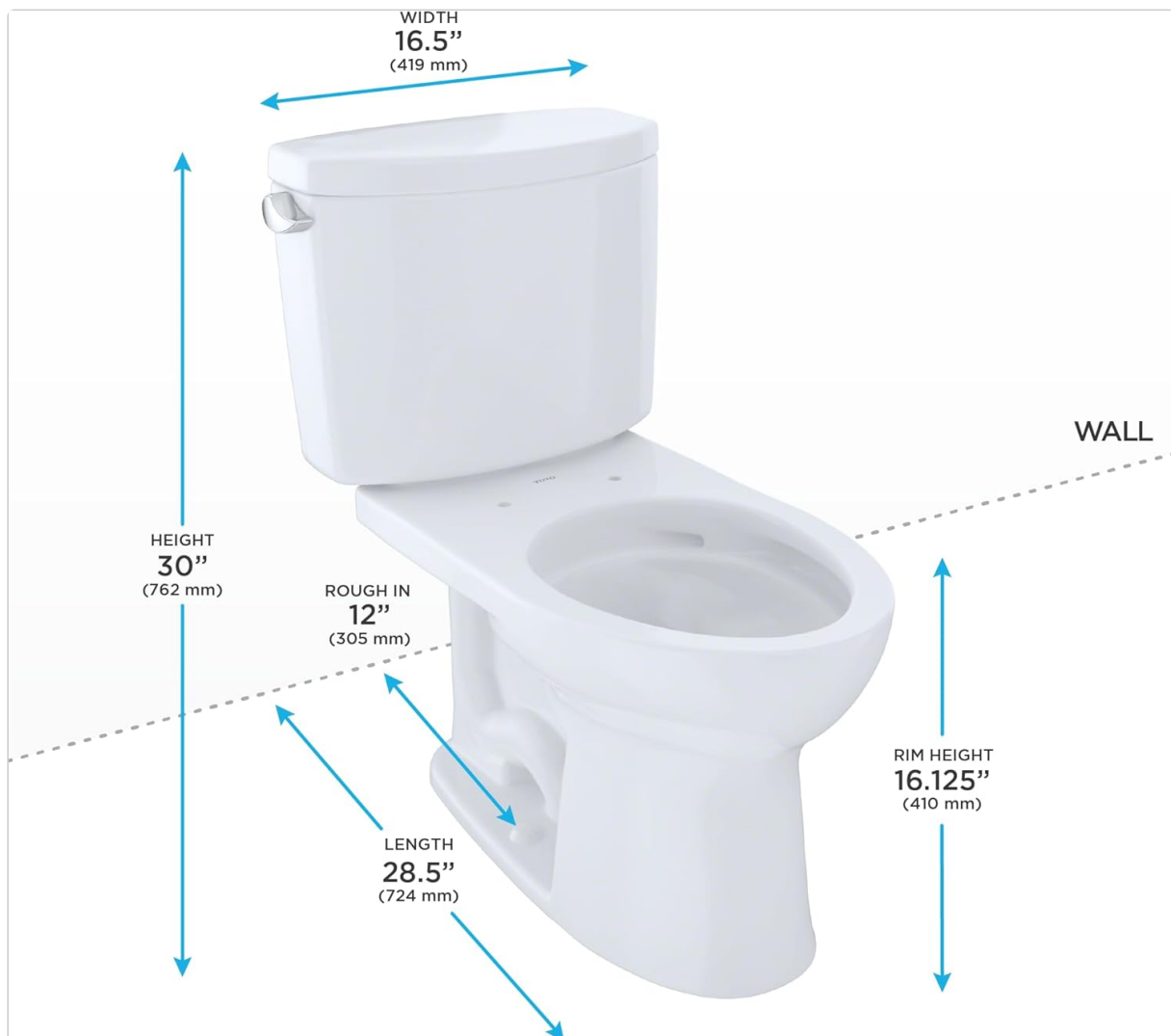
Dimensional diagram of the TOTO Drake II toilet, including height, width, length, rim height, and 12-inch rough-in.
