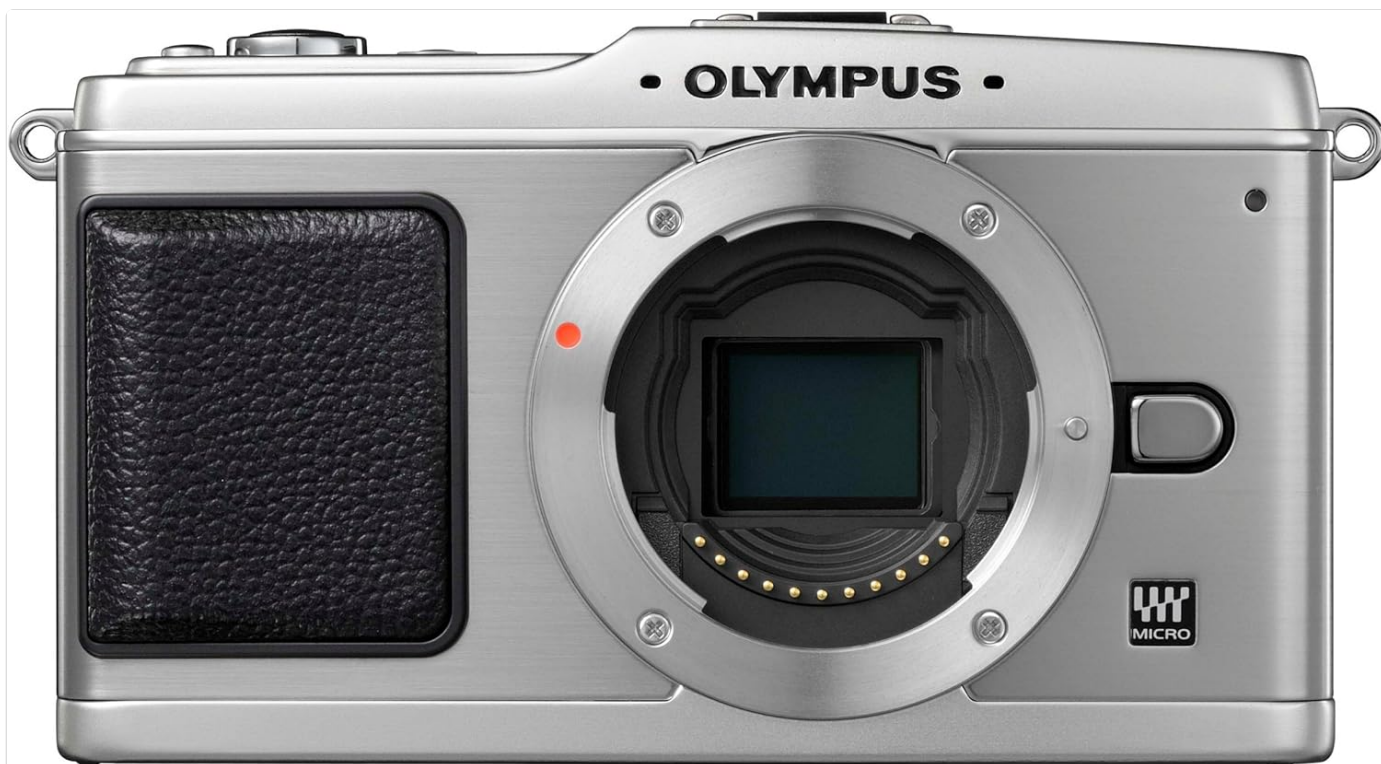
Figure 2: Front view of the Olympus PEN E-P1 camera body, illustrating the Micro Four Thirds lens mount.
