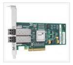
An image showing the HP 42B PCIe 4GB FC Dual Port HBA, a green circuit board with two Fibre Channel ports and a PCIe connector.
