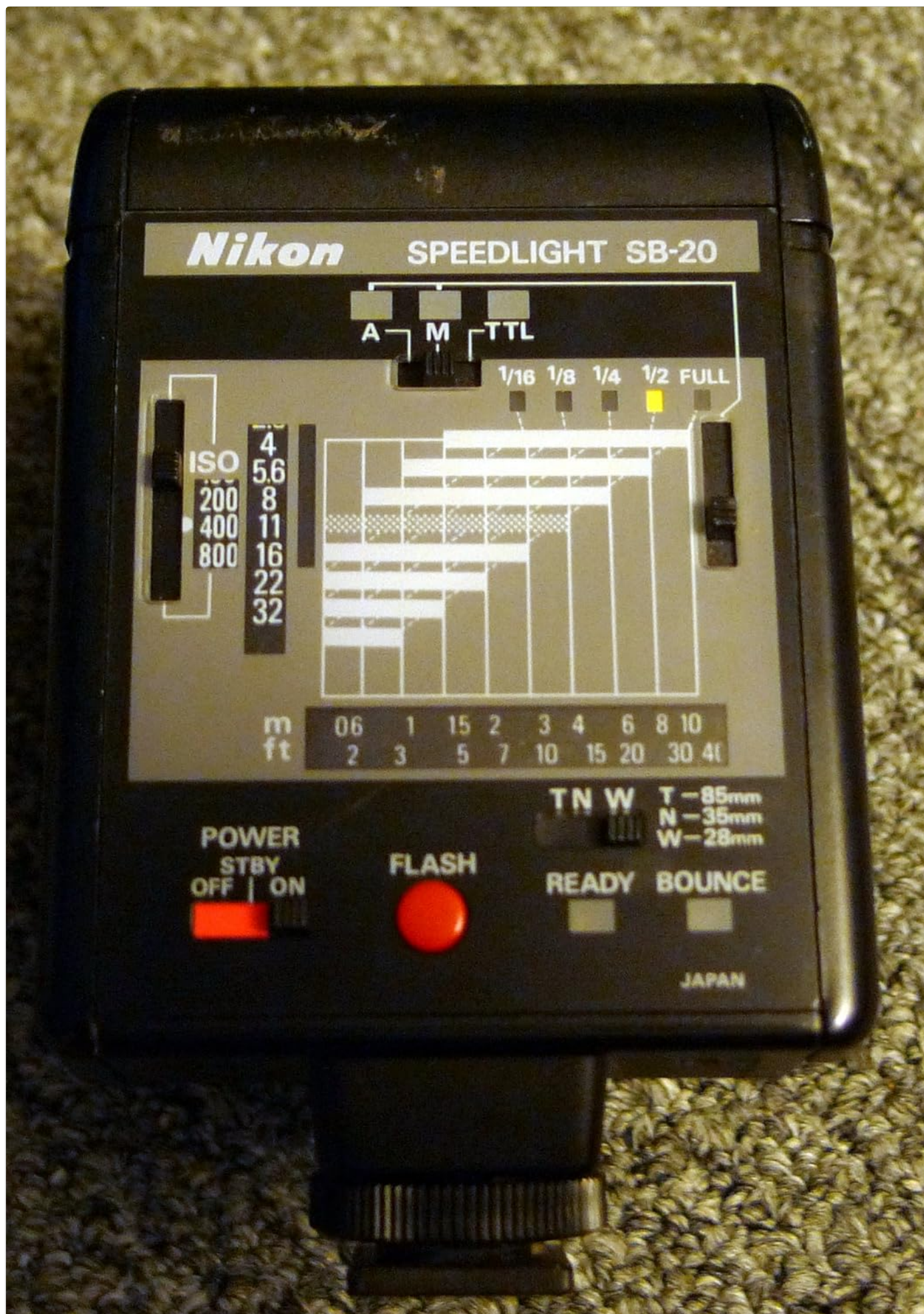
Figure 3: Detailed view of the SB-20 Speedlight's control panel, including the power switch and mode settings.
