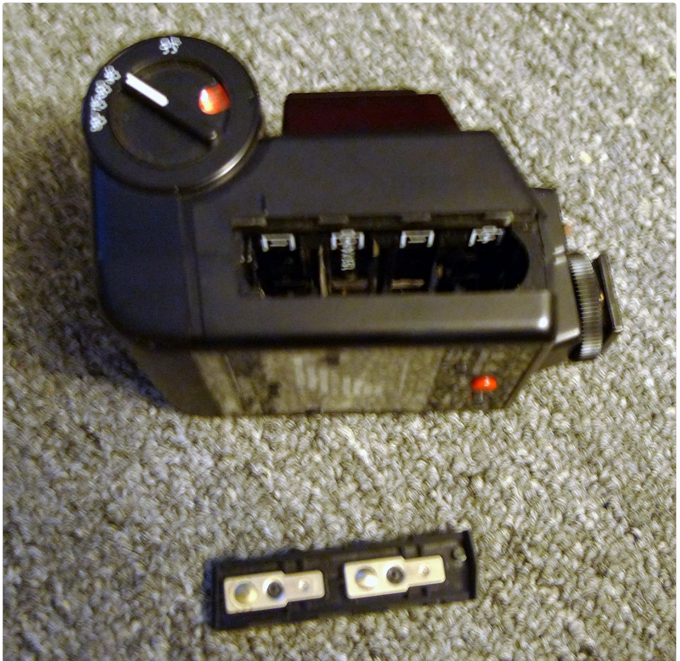
Figure 1: Open battery compartment of the SB-20 Speedlight, showing the slots for four AA batteries and the removable battery tray.
