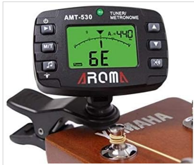
Image: The AMT-530 display showing tuner mode, indicating a note and the A4 reference pitch, clipped to a guitar headstock.
