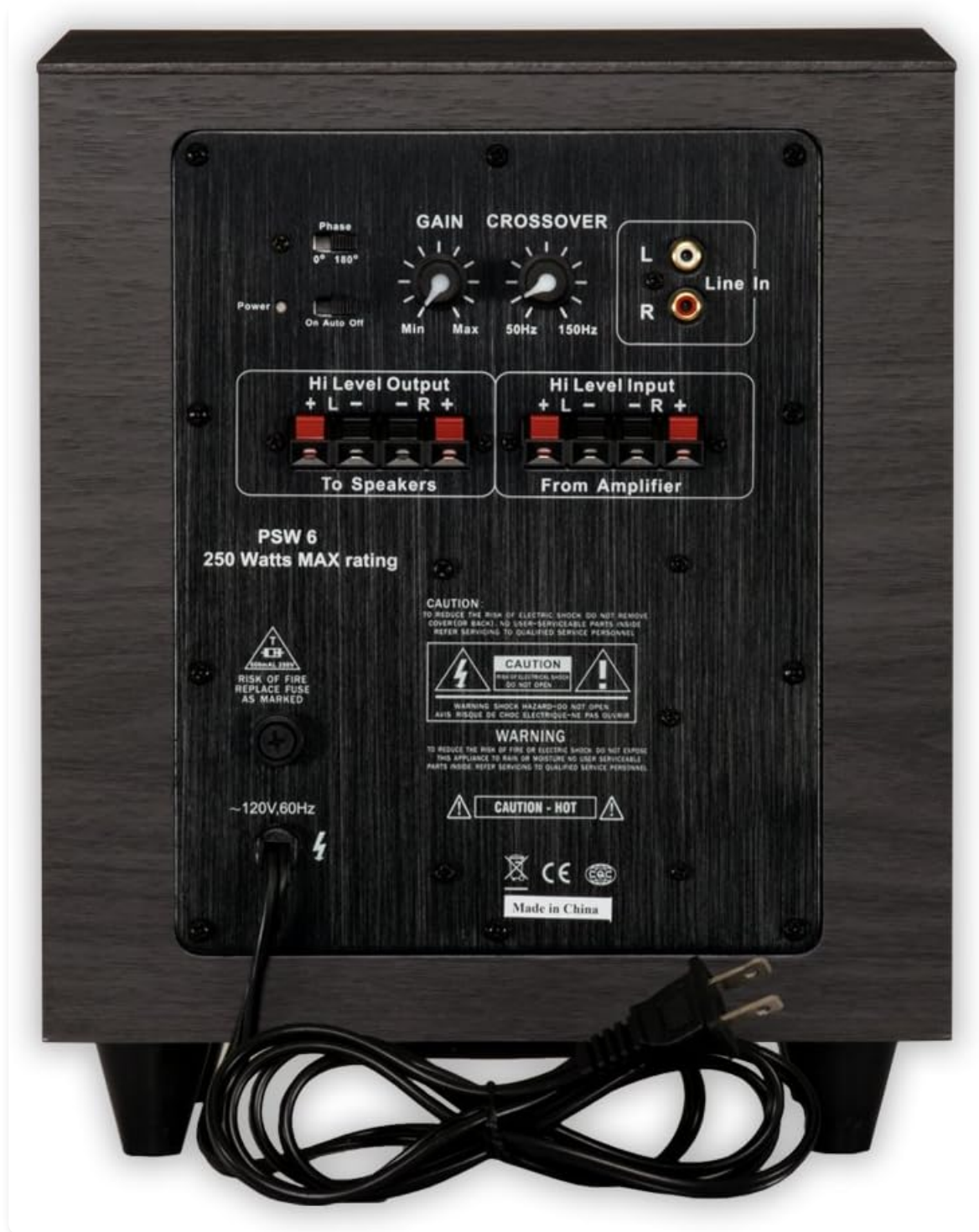
Figure 3: Rear panel connections and controls of the PSW-6 subwoofer.
