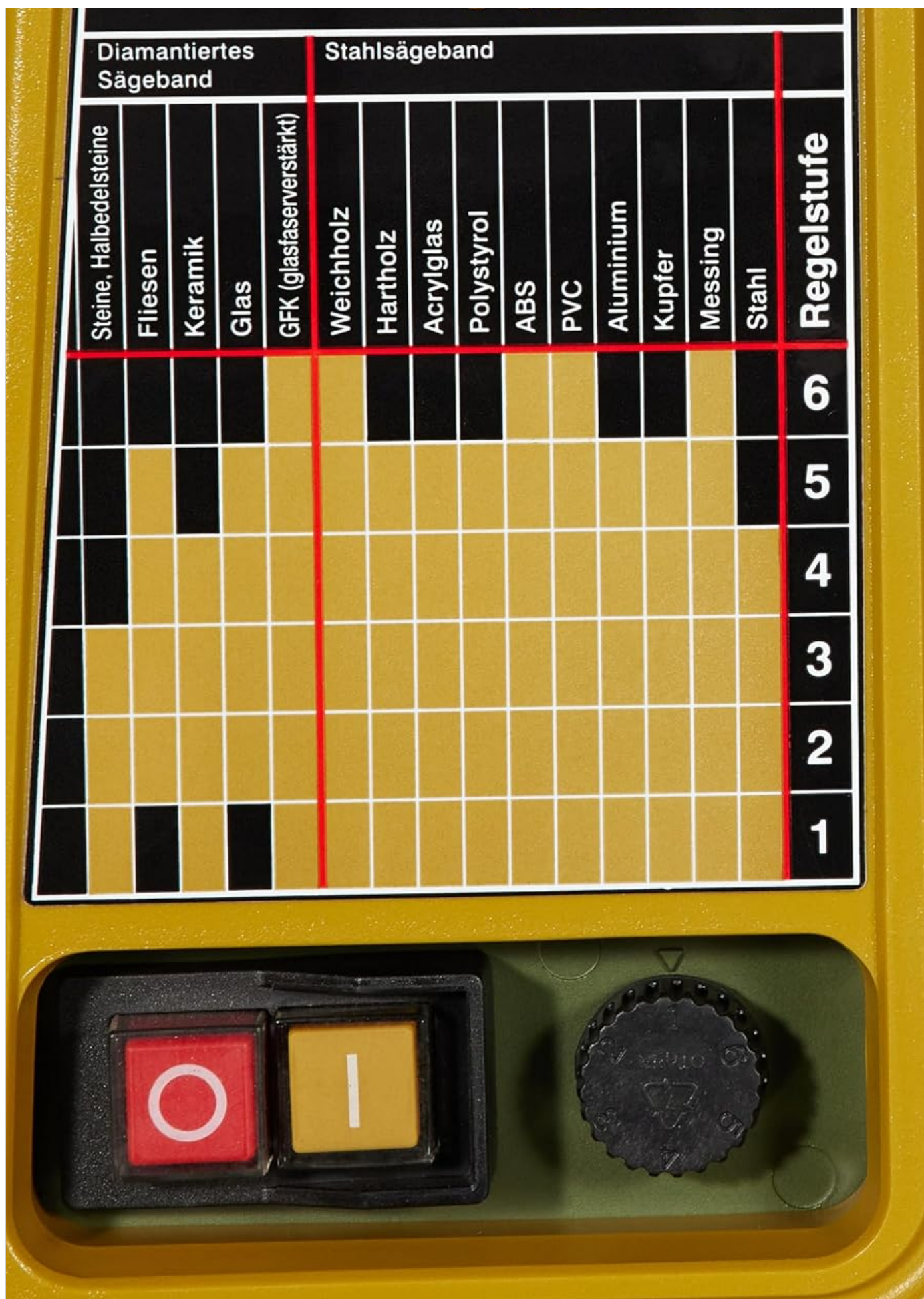
Figure 4: Integrated material cutting guide chart on the machine, providing recommendations for various materials and blade types.
