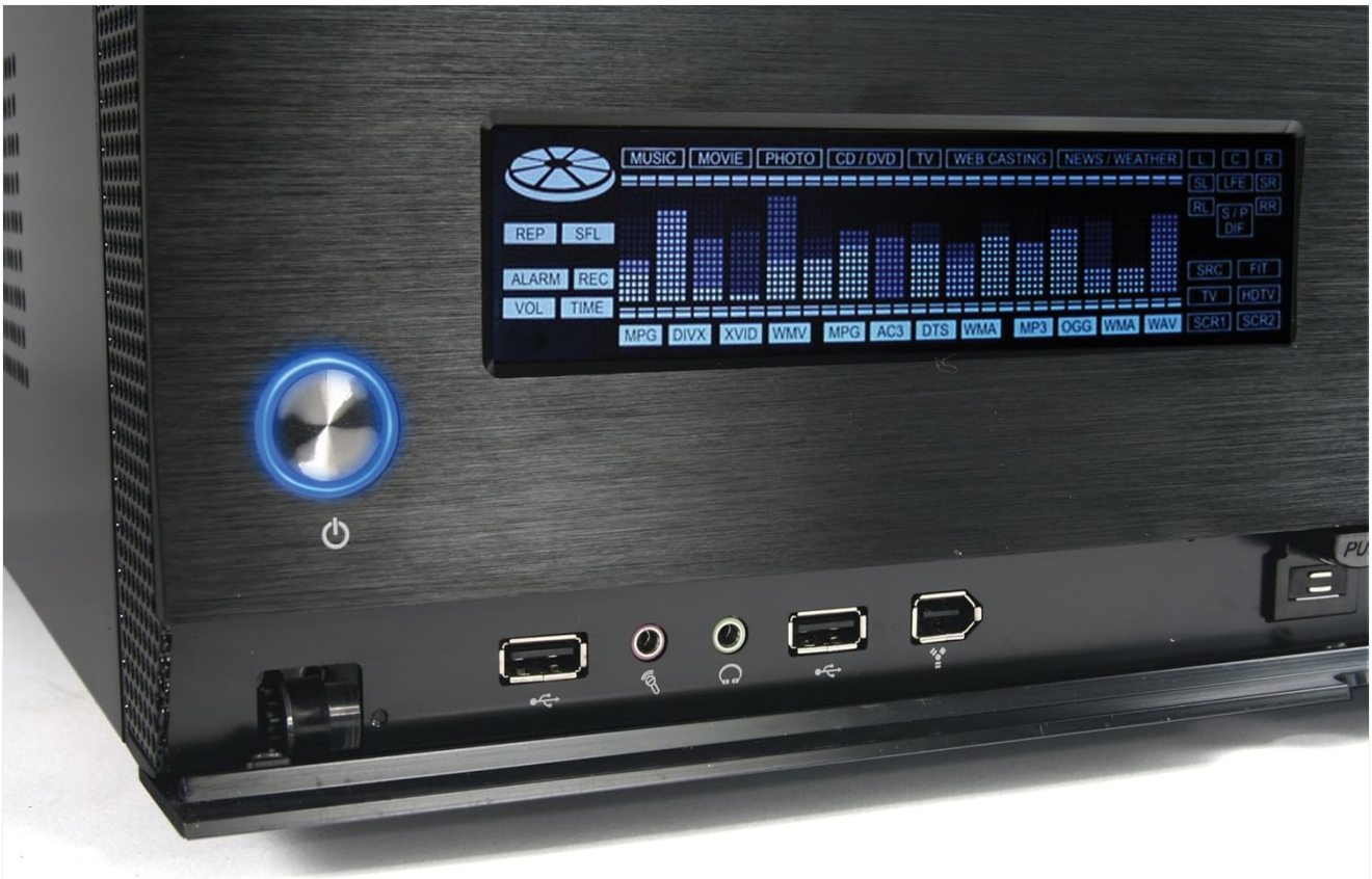
Figure 2: Detailed view of the front panel, highlighting the Media LAB LCD screen, two USB 2.0 ports, IEEE 1394 Firewire port, HD Audio jacks, and the 23-in-1 card reader slot.
