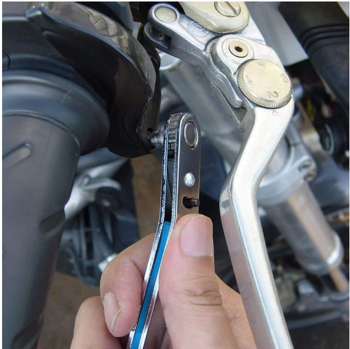
Figure 5.1: Demonstrating the screwdriver's ability to access screws in extremely tight and confined areas.
