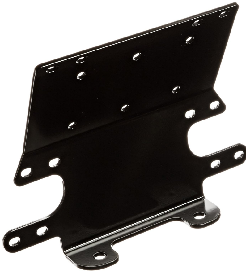
Figure 1: KFI Products 100545 Winch Mount. This image displays the black, powder-coated metal winch mount from an angled perspective, highlighting the various pre-drilled holes for winch and fairlead attachment, as well as the U-bolt mounting points for securing it to the ATV frame.
