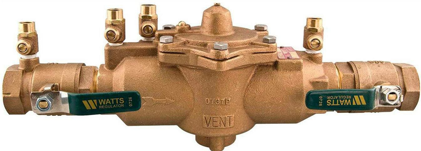
Figure 1: Watts 009M2 Reduced Pressure Zone Backflow Preventer. This image shows the bronze body, quarter-turn shutoff valves with green handles, and multiple test cocks on top.
