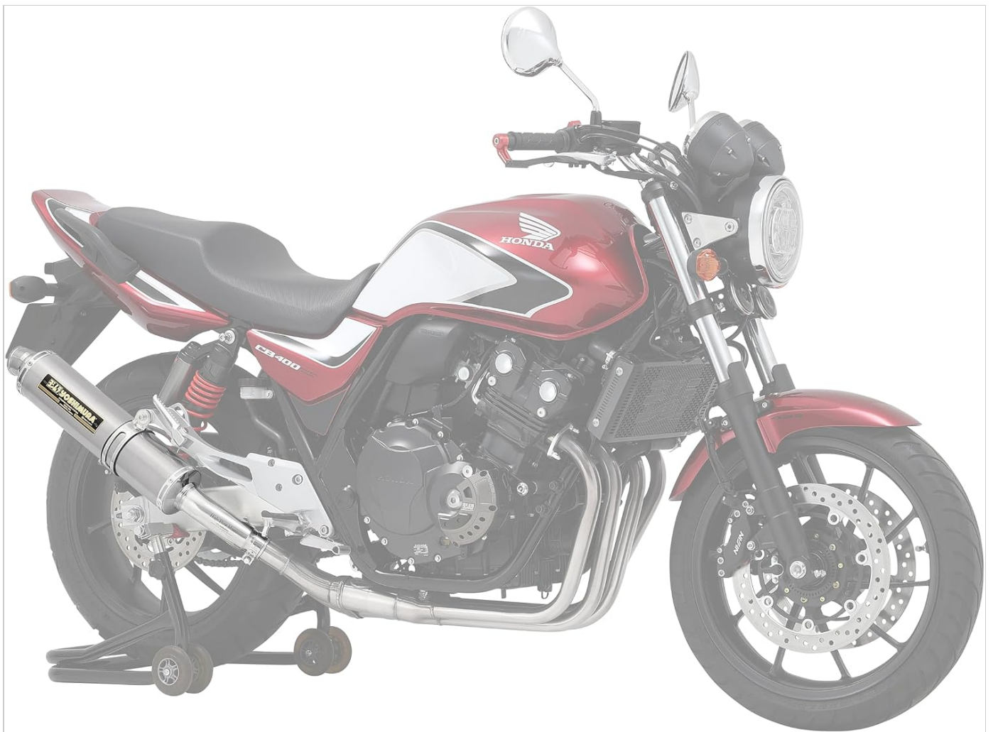
Figure 3.1: Yoshimura Slip-On Exhaust System (Stainless Steel) installed on a Honda CB400SF.
