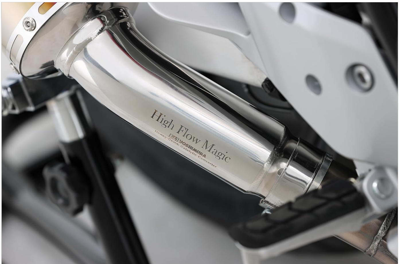
Figure 3.1: Yoshimura Slip-On Exhaust System (Stainless Steel) installed on a Honda CB400SF.
