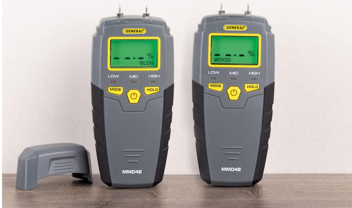
Figure 3: The moisture meter displaying "BLDG" for building materials mode and "WOOD" for wood mode, illustrating the dual functionality.
