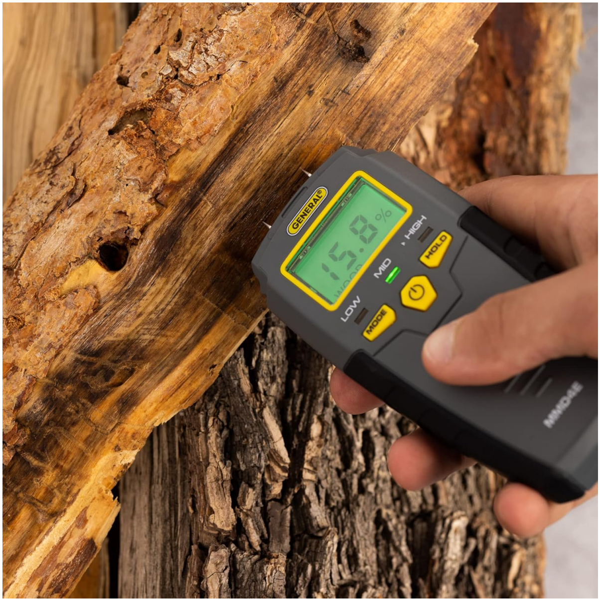
Figure 4: A hand holding the moisture meter, with its pins inserted into a piece of wood, displaying a moisture reading on the screen.
