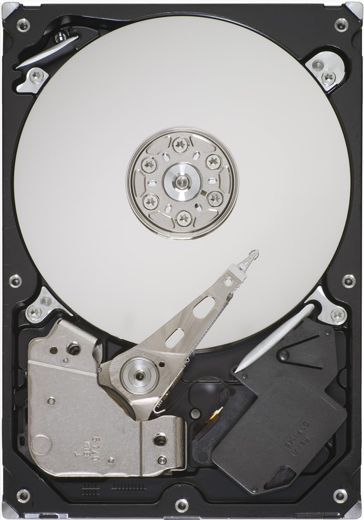
Figure 1: Internal view of a Seagate Barracuda 7200 1 TB hard drive. This image displays the internal structure of the Seagate Barracuda 7200 hard drive. Visible components include the shiny circular platter where data is stored, the read/write head arm positioned over the platter, and various electronic and mechanical parts that facilitate data access and storage.
