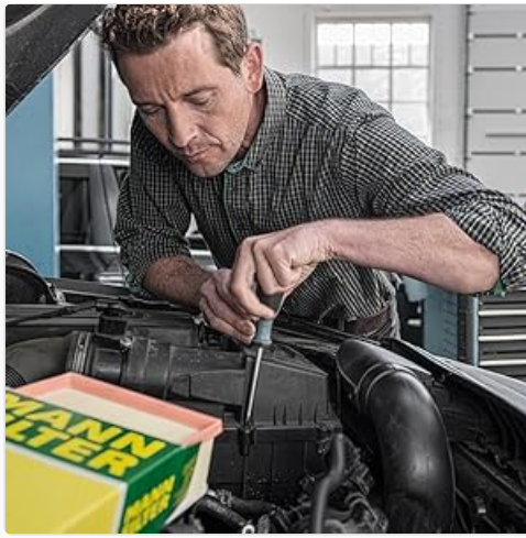
Image 3.1: A mechanic installing an air filter, demonstrating a typical installation scenario.
