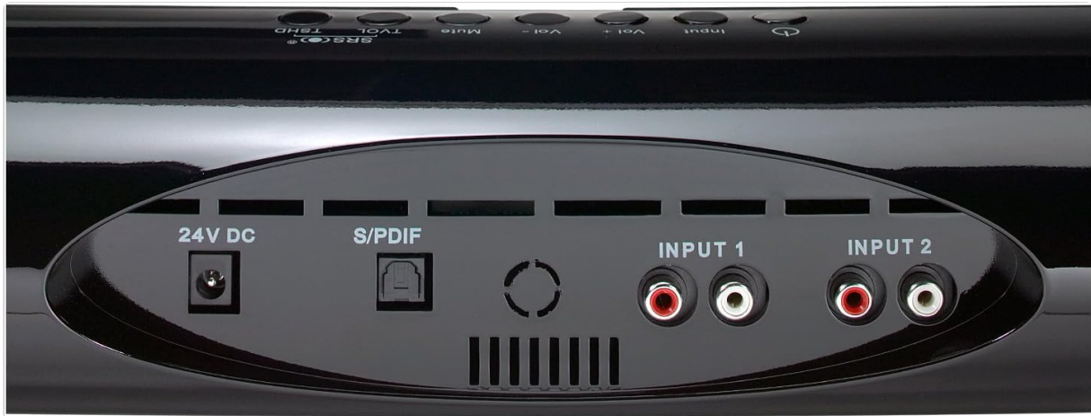
Image: Rear panel of the VSB210WS Sound Bar, displaying the 24V DC power input, S/PDIF optical input, and two sets of RCA analog inputs (INPUT 1 and INPUT 2).
