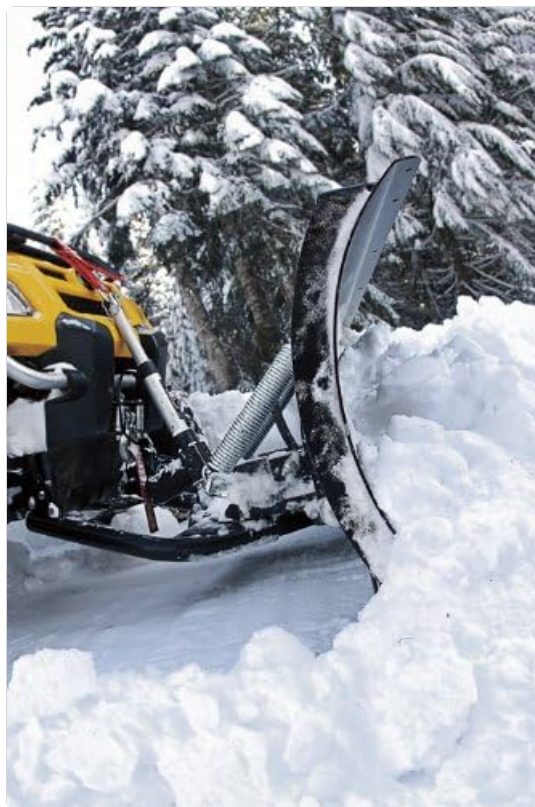
Figure 3: WARN plow mount installed on an ATV with a snow plow.
