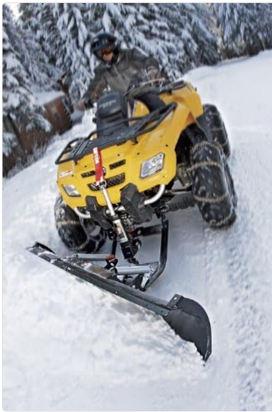
Figure 4: ATV demonstrating the front-mount plow system in a raised position.
