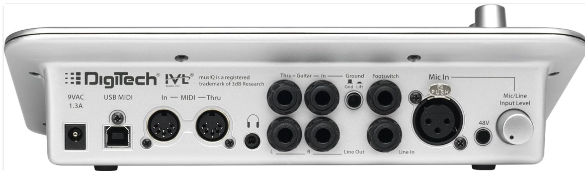
Image: Rear panel connections of the Vocalist Live 3D.
