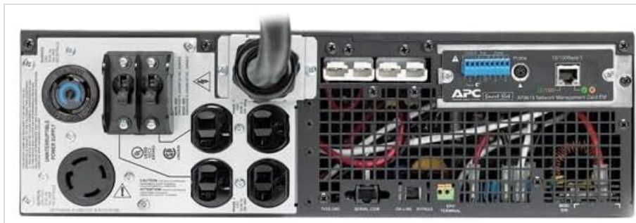
Figure 3.2: Rear view of the APC Smart-UPS RT 5000VA. This image displays the rear panel of the APC Smart-UPS RT 5000VA, highlighting various power outlets including NEMA L6-20R, NEMA L14-30R, and NEMA 5-20R receptacles, along with communication ports for network management and serial connections. The main power input cable is also visible.
