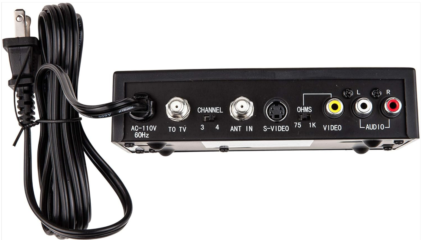
Figure 2: Rear panel of the Steren 203-101 RF Modulator, displaying the AC power input, TO TV (RF output), ANT IN (RF input), CHANNEL 3/4 switch, S-VIDEO input, VIDEO (composite) input, and AUDIO L/R (stereo) inputs.
