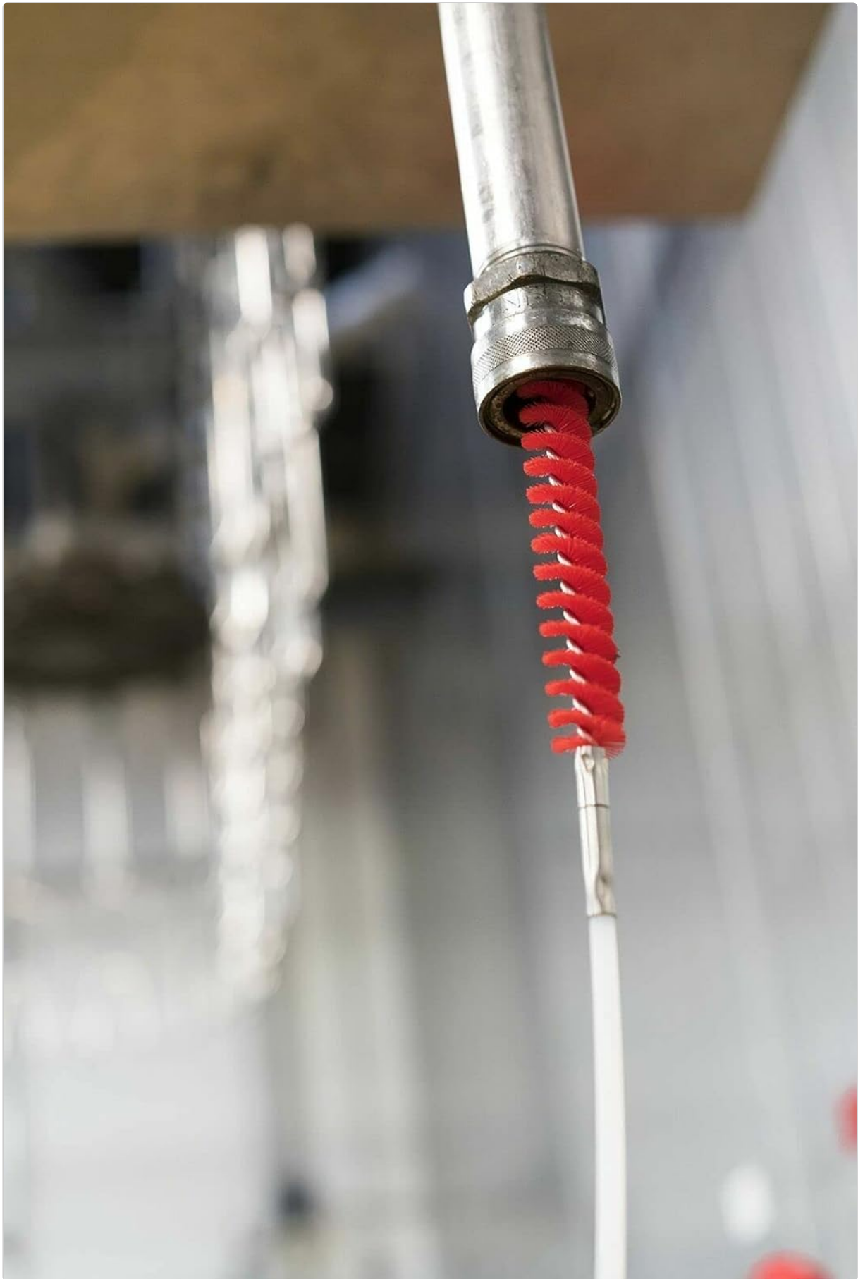
Figure 1: The Vikan 53603 Tube Brush shown attached to a flexible handle, ready for insertion into a pipe. This demonstrates the secure connection point between the brush and an extension handle.
