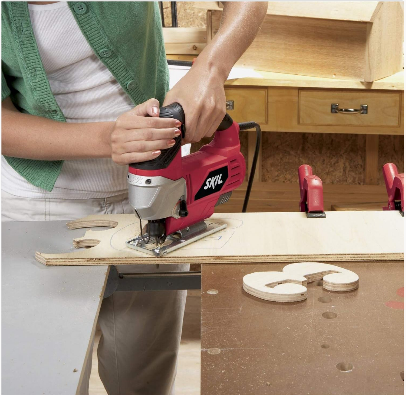
Figure 3: Cutting a curved shape. Use a narrow blade and a lower orbital setting for best results.
