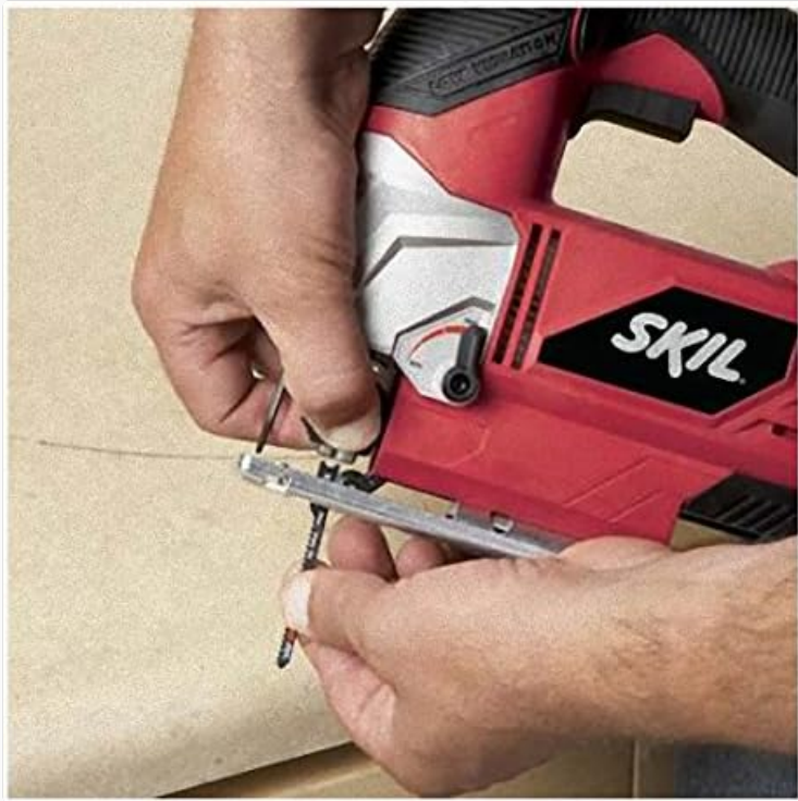
Figure 1: Installing the blade. Ensure the jigsaw is unplugged before changing blades.
