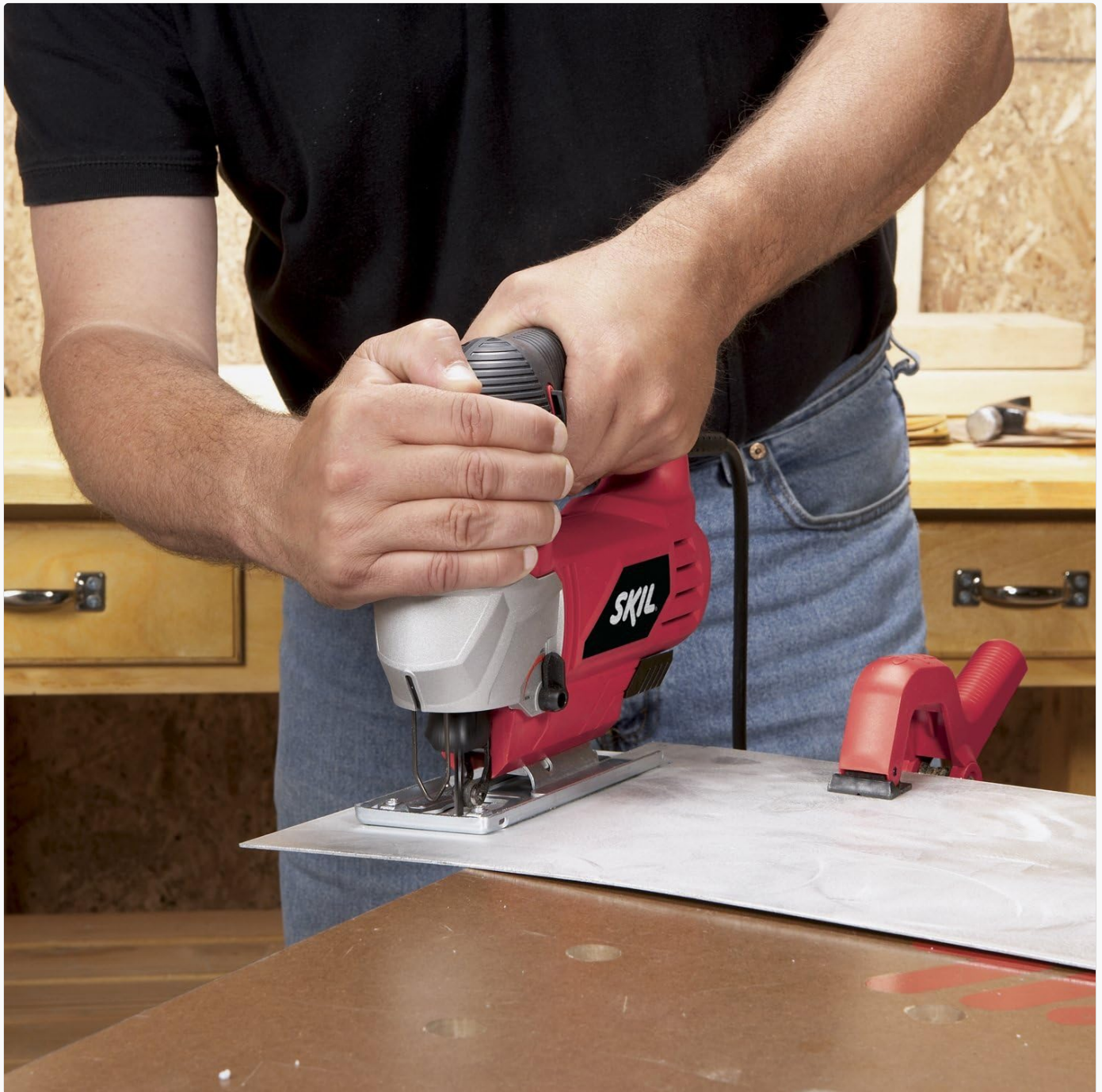
Figure 2: Performing a straight cut with the jigsaw. Maintain a firm grip and steady pressure.
