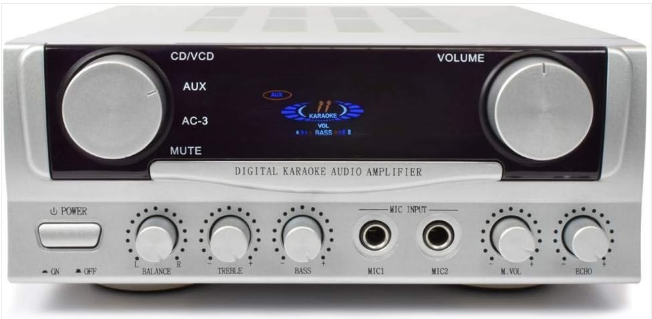
Figure 1: Front Panel Layout. This image displays the amplifier's front panel, highlighting the power button, input selection knob, volume control, microphone inputs, and tone controls.
