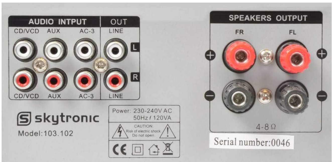
Figure 2: Rear Panel Connections. This image illustrates the various audio input and output ports, including RCA inputs, line output, and speaker terminals.
