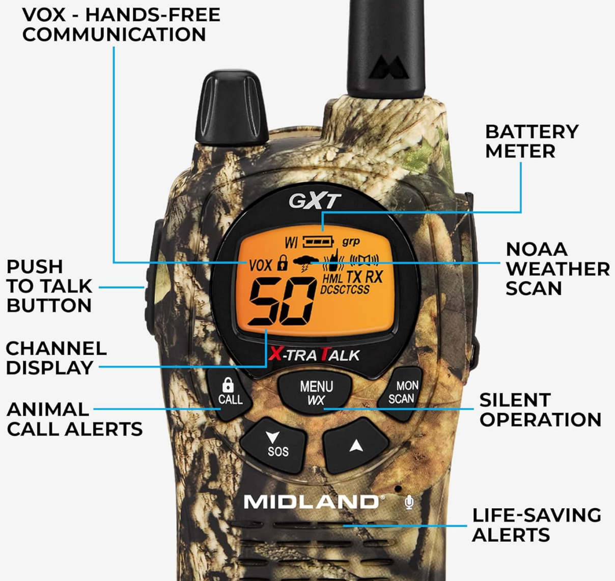
Image: Diagram illustrating the various controls and display elements of the Midland GXT1050VP4 radio, including the Push-to-Talk button, Channel Display, VOX indicator, Battery Meter, NOAA Weather Scan, Animal Call Alerts, Silent Operation, and SOS button.
