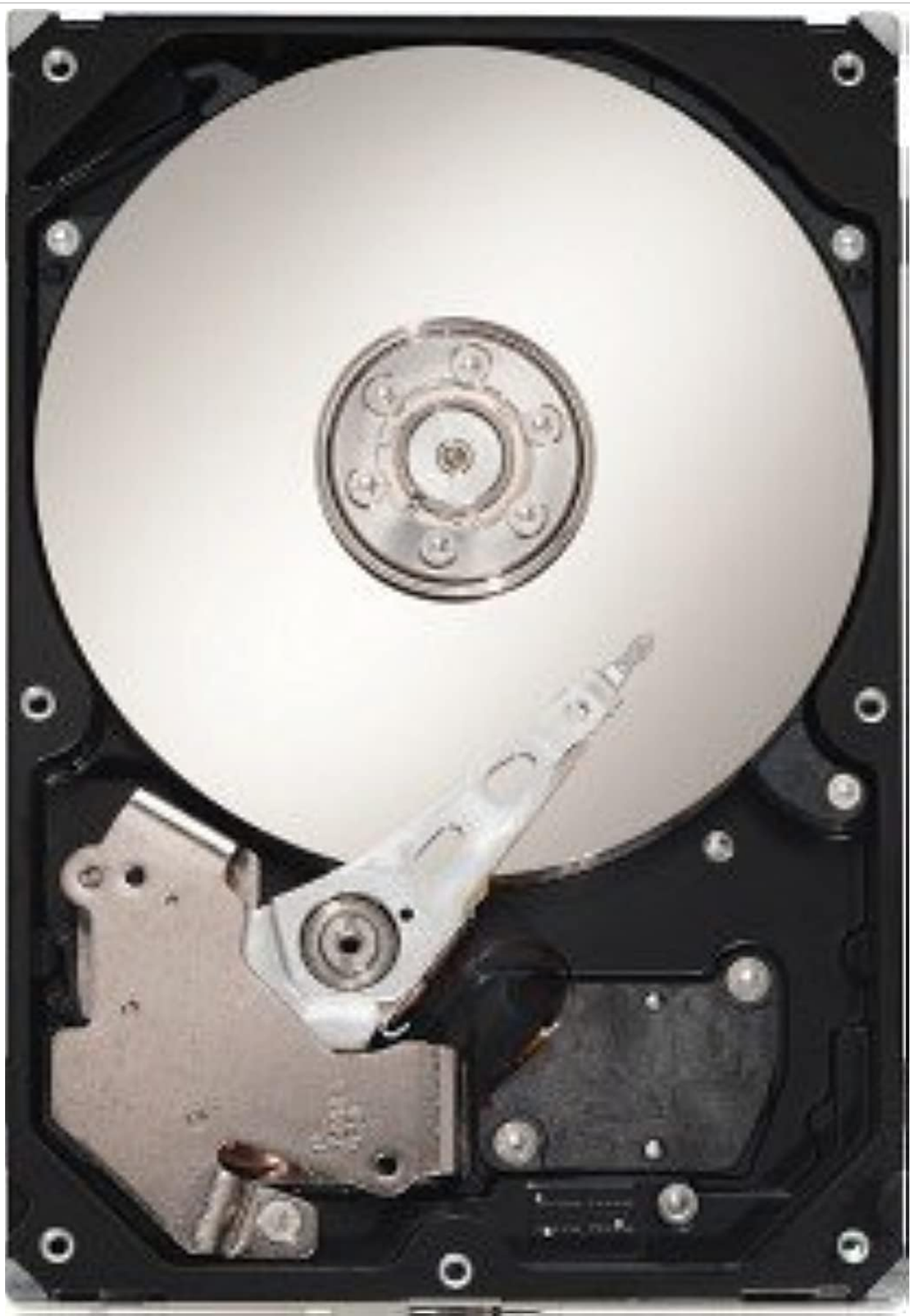
Figure 2.2: View of the internal components of a Seagate Barracuda hard drive, illustrating the platter and read/write head mechanism.
