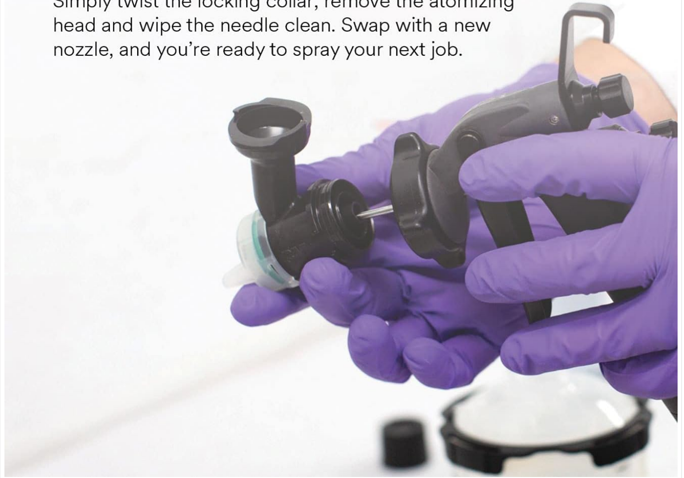
Image: Hands demonstrating the quick removal of the atomizing head by twisting the locking collar, followed by wiping the needle clean, illustrating the "Cleans in Seconds" feature.
