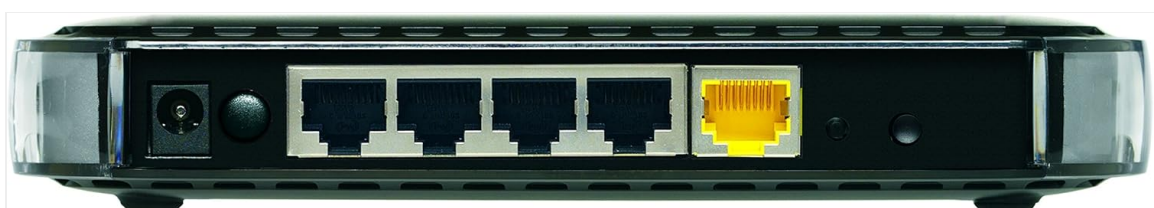
Image: Rear view of the NETGEAR WNR1000-100NAS router, displaying the power input, four yellow LAN ports, and one blue WAN/Internet port.
