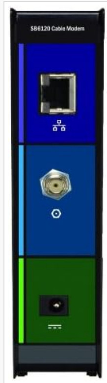
Image: Rear view of the Motorola SB6120 cable modem, highlighting the Ethernet port (top), Coaxial cable connector (middle), and Power input (bottom).
