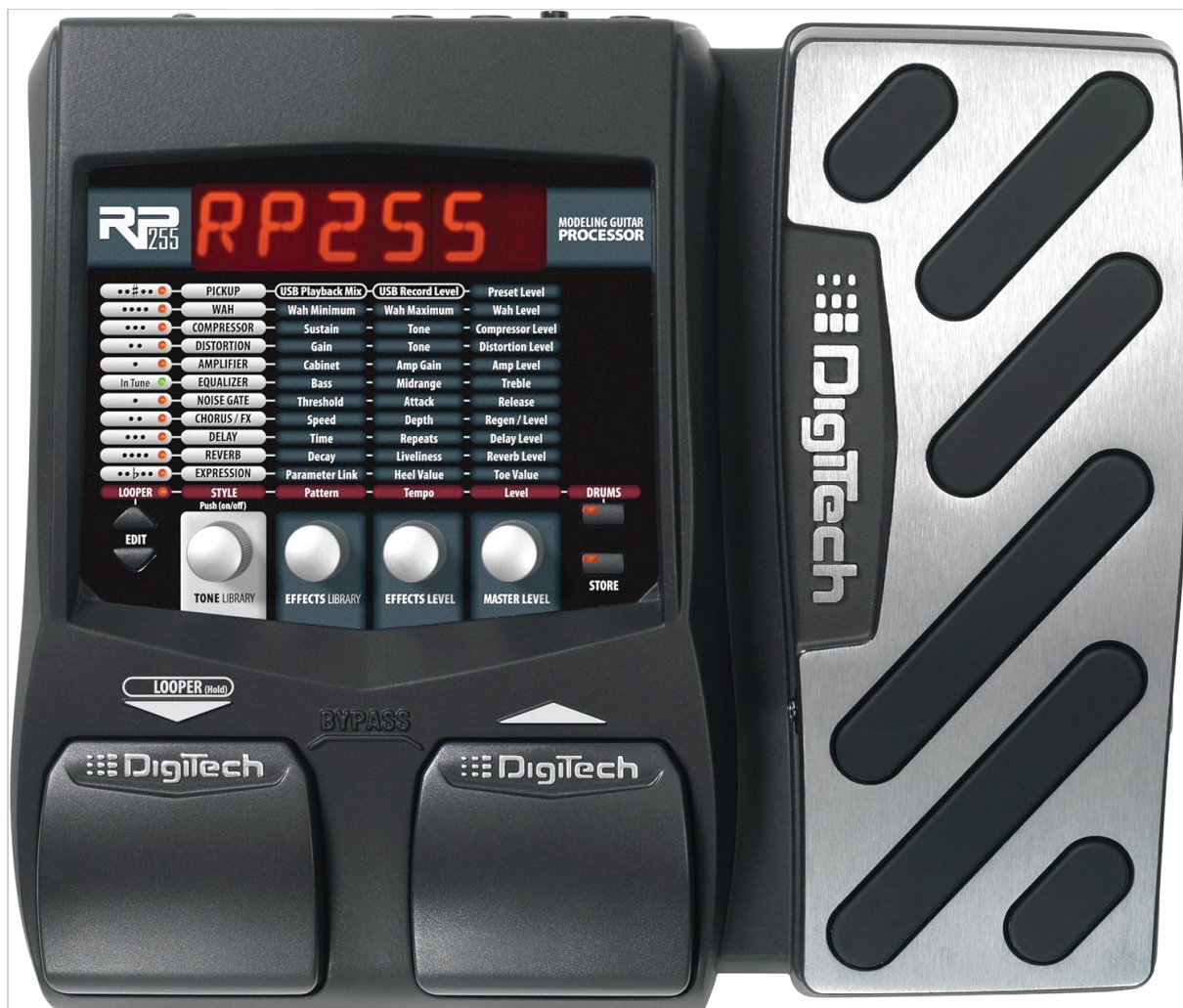
Figure 1: Front view of the DigiTech RP255, showing the display and control pedals.
