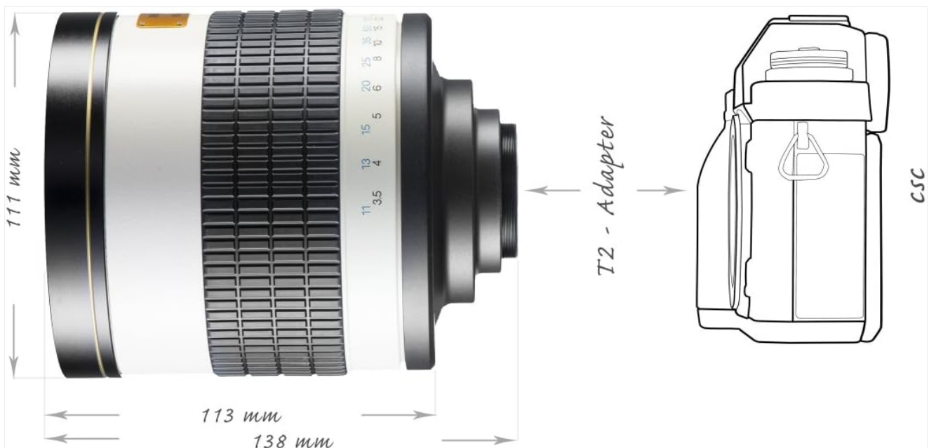
Image Description: A diagram illustrating the Walimex Pro 800mm lens connected to a DSLR camera (SLR) via a T2 adapter. The lens dimensions (111mm height, 113mm length, 138mm total length with adapter) are indicated.
