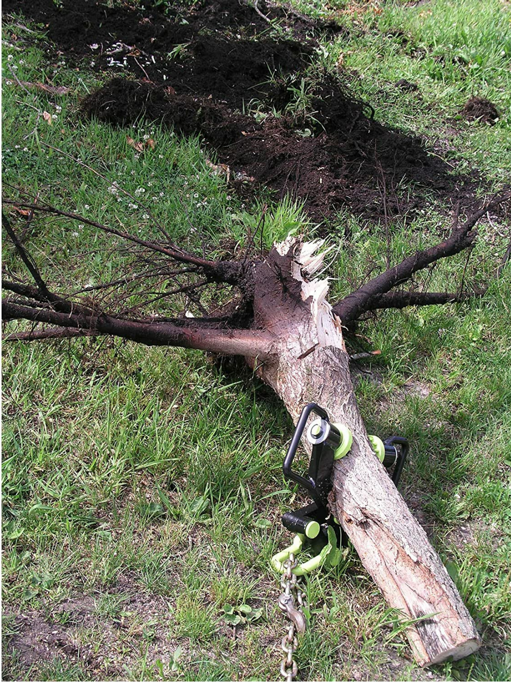
Figure 4: A tree stump successfully removed from the ground, with the Brush Grubber BG-11 still attached.
